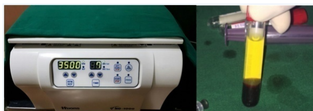
Fig. 1: Centrifuge first spin: 3500RPM x7 minutes
